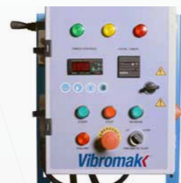
Electrical Control Panel
